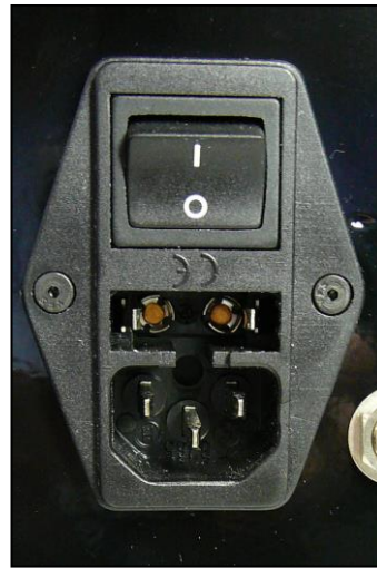
FUSE HOLDER REMOVED
